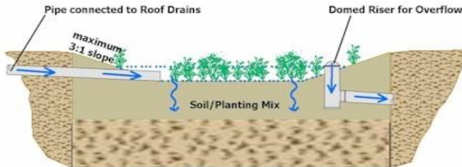
Typical Rain Garden/Bioretention Area
